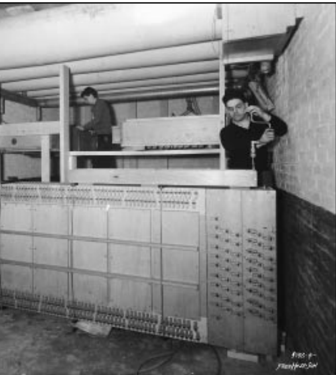
combination action. Sadly, this precision-made equipment was nearby pipes carrying steam and hot water upset its delicate mechanism was ruined by the hurricane of 1944 which flooded the shop where this equipment is housed.
