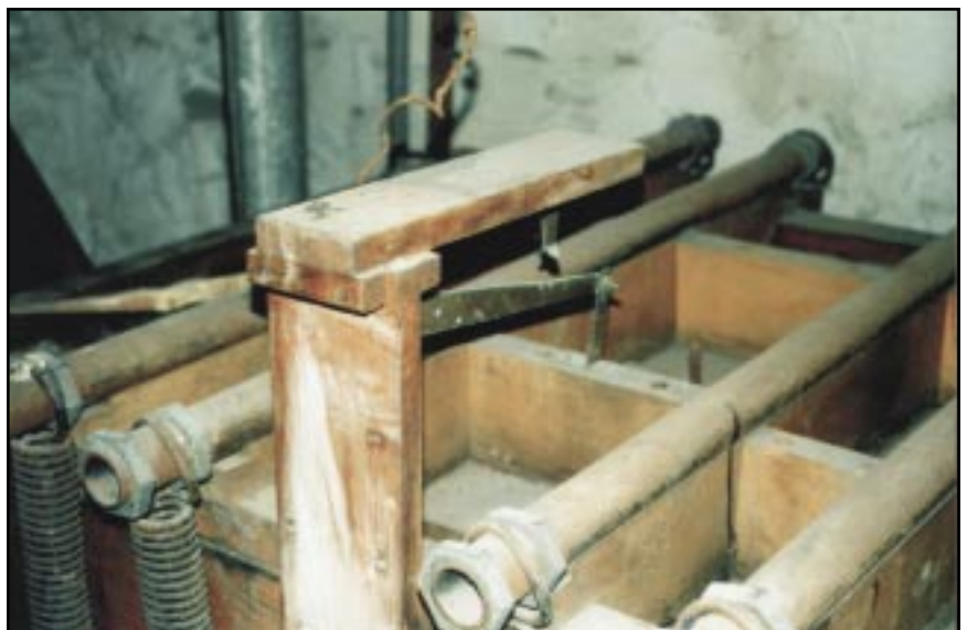
Wind regulator for the Gallery I organ's 100-inch reeds. Eight springs on the sides of this device exert some 3,000 pounds of pressure and the knife switch (seen at top) only makes contact — allowing the stops to speak — when the full pressure is reached.
