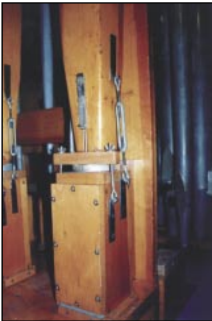
Heavy duty construction! Turnbuckle mechanisms secure the various parts of the 100-inch Grand Ophicleide's 16-foot pipe. Note, also, the bracket that holds the tuning wire in place.
