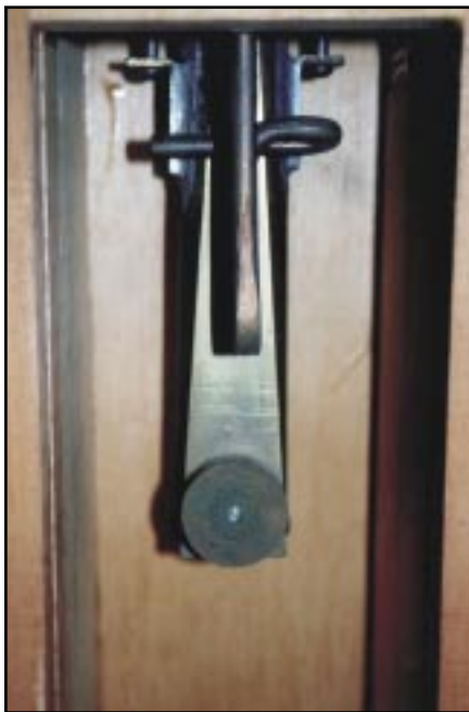
Heavy duty construction! The tuning wire and weighted tongue of the 100-inch Grand Ophicleide's 16-foot pipe.
