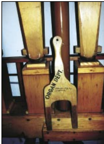
Wooden wrench used to lift Diaphone pipes
