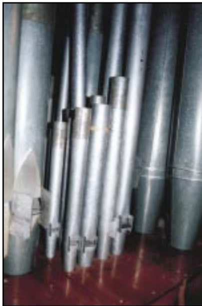
The Solo organ's four-rank Carillon mixture. Note the combination of open, capped, and harmonic ranks. On the picture's right, are some Wald Flute pipes with two solder lines — indicating that the second (double) languid was inserted after the pipes were originally made in the normal way. On the left, a couple of Tibia Rex pipes, with their very large ears, can be seen.
