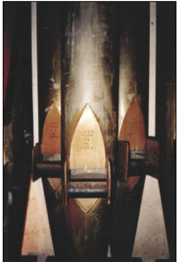
Some of the larger pipes in the Choir organ's Dulciana rank. Stamped above the upper lip on the center pipe are: “171” (stop number), “5550” (Midmer-Losh opus number), “16” (pitch), “DUL” (Dulciana), “AAA#” (note).
