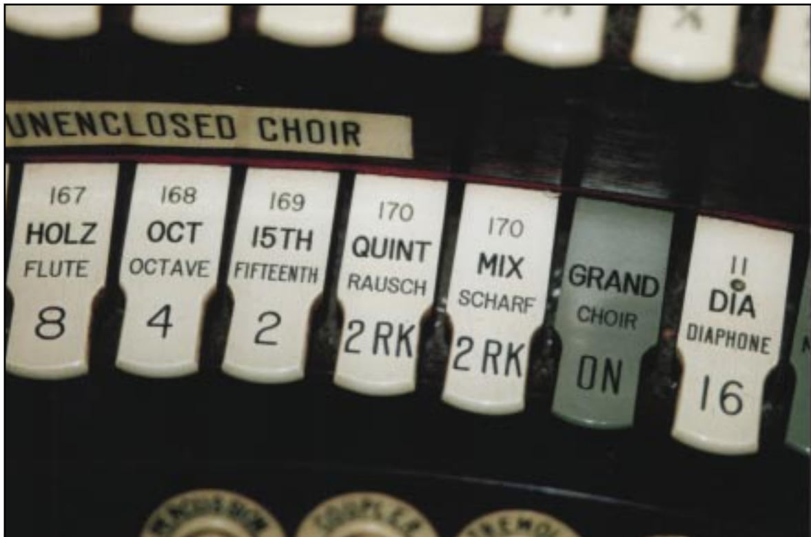
A view showing most of the Unenclosed Choir organ's stop-keys on the main console. Note how the department's four-rank mixture, stop #170, is operated by two registers (Rausch Quint and Scharf Mixture), each controlling two ranks. How well do you know the Convention Hall organ? Can you identify the two registers belonging to the Unenclosed Choir that aren't viewable in this picture?
