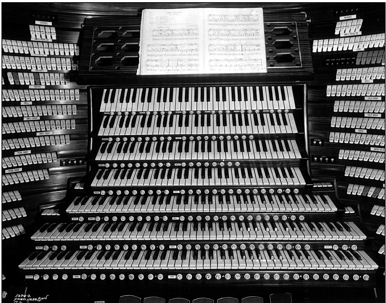
Main console – front view, showing the pistons, indicators (at sides of Fanfare manual), and rocking tablets (adjacent to Solo and Fanfare manuals).
