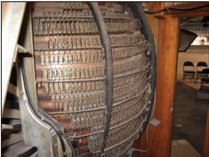
View behind the 7-manual console showing stop tab wiring and angles of the seven keyboards.
