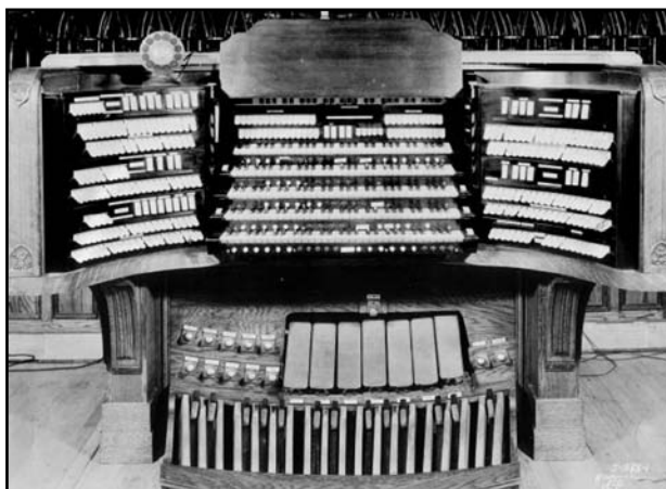
The five-manual console. The vertical stop-keys were couplers. The swell shoes, from left to right, were for: Antiphonal, Great, Solo (and Pedal), Orchestral, Floating, and Choir. The far-right shoe was the General Crescendo and the foot piston above the center shoe (Orchestral) switched all shades onto that shoe.
