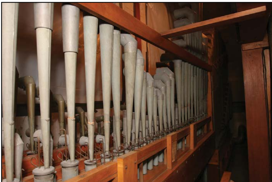
100-inch reeds in the Gallery I organ. Nearest the camera is the Tuba Maxima — the first stop in the world to be voiced on this extreme pressure.
