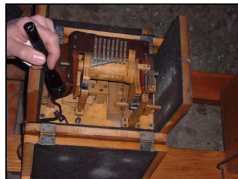
The shade control that is part of the roll player mechanism. This device is on the bottom left of the relay rack. Photo by Harry Bellangy
