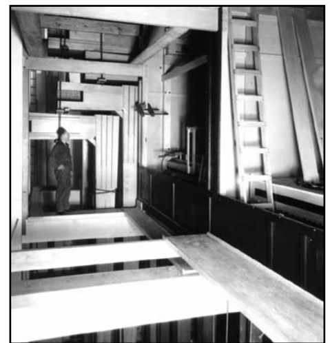
Dulzian pipes and Great-Solo swell boxes. The man seen here is standing next to the GGGGG# pipe, and the CCCCC and CCCCC# pipes (not visible) pass through the rear of the swell box (furthest from camera) containing the Orchestral division of the Great-Solo (the swell box nearest the camera is for the Great-Solo’s flues). The space in front of these swell boxes is now occupied by the Great organ’s chests.
